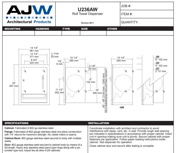
**Towel Dispenser:** Mechanism is fabricated of high impact plastic and #20 gauge steel has a capacity for one standard roll and one stub roll. Lever can be operated with one hand and less than 5 lbs of force to comply with ADA code. Mechanism has three settings to adjust for desired towel lengths.
