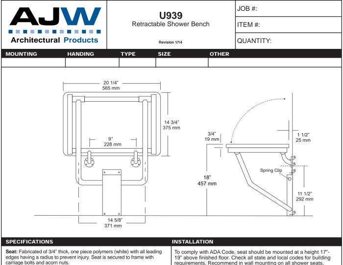
Tubing: Fabricated of #18 ga stainless steel with #4 satin finish.
