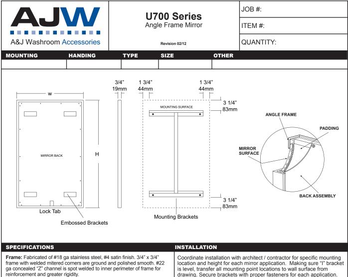
**Mirror:** 1/4" thick type 1 transparent flat type, class 1 - clear glass mirrors. Mirror is coated with silver and sealed with a uniform electrolytic copper plating, along with two coats of paint for added protection. Mirrors are guaranteed against silver spoilage for a period of 15 years. Mirrors conform to ASTM C1036 and ASTM C1503-R8.
