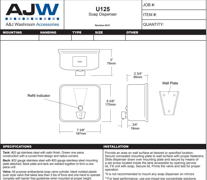
**Refill Indicator:** Clear plastic viewer window allows a constant fluid level check.
