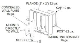
All UX bath accessories series are fabricated of type 304 stainless steel with a bright finish. Mounting plates are concealed with a snap-on type plate secured by a set screw.
