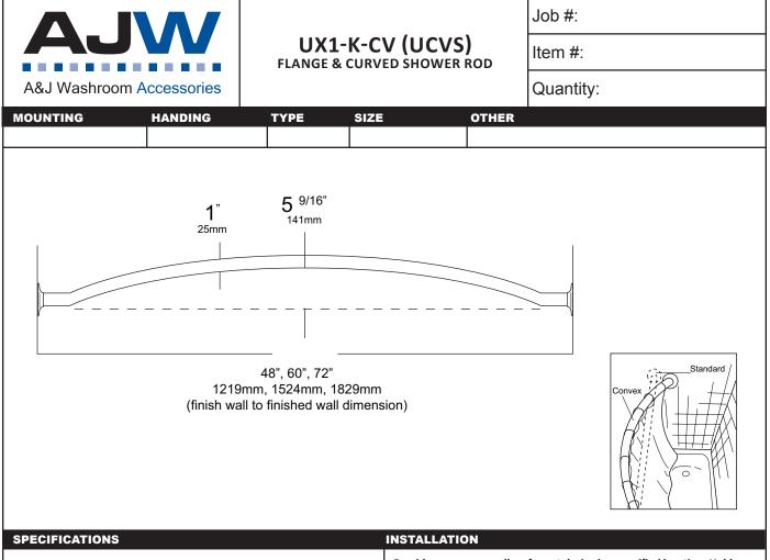
**Rods:** Fabricated of type 304 stainless steel with a #4 satin finish with a 1" outside diameter. Rod configuration is accomplished by a roll former that provides an additional 5 9/16" showering area. (Aprx. 25%)
