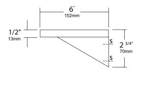
**Shelves**: Type 304 #18 ga stainless steel. All edges are turned down 1/2" with front edges turned down & back 1/2" for maximum strength and rigidity. All corners are deburred and polished smooth for safety.
