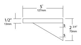
**Shelves**: Type 304 #18 ga stainless steel. All edges are turned down 1/2" with front edges turned down & back 1/2" for maximum strength and rigidity. All corners are deburred and polished smooth for safety.
