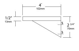
**Shelves**: Type 304 #18 ga stainless steel. All edges are turned down 1/2" with front edges turned down & back 1/2" for maximum strength and rigidity. All corners are deburred and polished smooth for safety.
